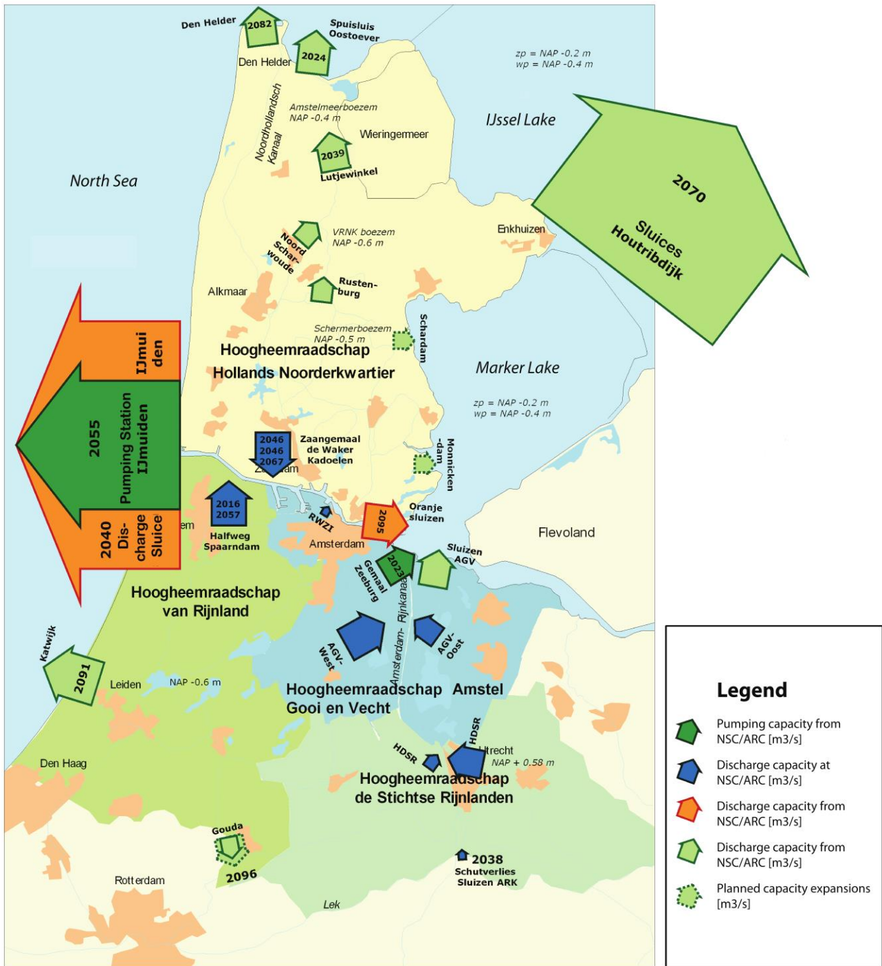
Figure 3. End of life predictions for hydraulic structure that are within the NSC/ARC network, as computed from the 'basic' method which utilizes founding year and design lifetime. Upper panel: a chronologic sequence of the resulting end of life predictions. Lower panel: a geographic representation.
