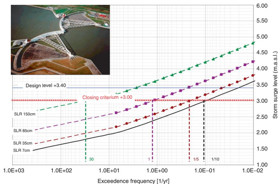
**FIGURE 4** | The storm surge barrier (Maeslantkering) to protect the Rotterdam Harbour and exceedance frequencies (per year) of water levels in the Rotterdam Harbour assuming a sea level rise between 0 and 150 cm (Reprinted with permission from Ref 24 Copyright 2008).
